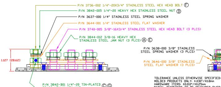
MOLDED PRODUCTS ONLY: ±.030"/±0.8mm HARDWARE ITEMS: ±0.010"/±0.25mm RADIAL DIAMETERS TO BE MEASURED OVER MANDRELS, RING GAGES OR PIN GAGES OF SUITABLE SIZE
