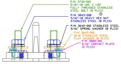
ALL DIMENSIONS GIVEN AS: in [mm] MOLDED PARTS: ±.030" [±0.8mm] HARDWARE ITEMS: ±.010" [±0.25mm]
